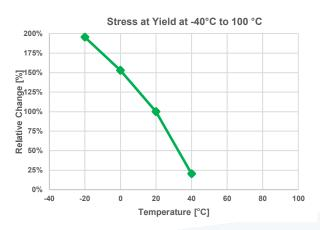
Test parameters: ASTM D638, Type IV, Pull speed: 50 mm/min, Young's modulus measured at 0.1-1% (regression),
